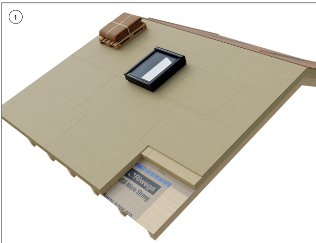
Place the pallet containing the folded membrane on top of the pitch to be covered
