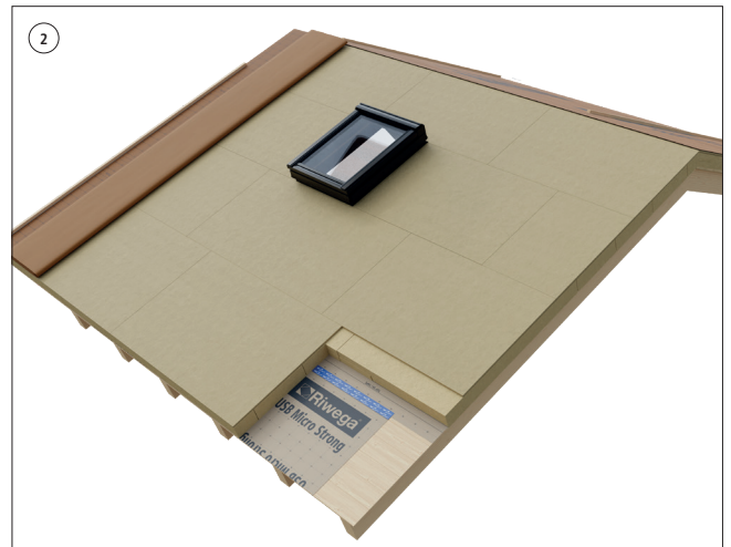
Unfold the membrane starting vertically and attach the first counter-batten to the edge of the pitch
