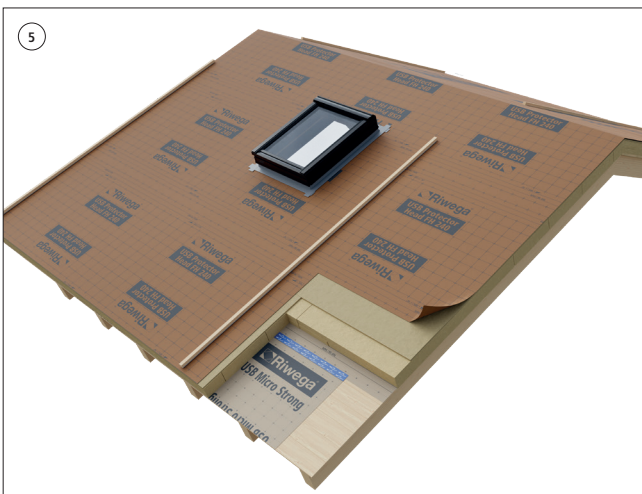
After laying the membrane on the roof pitch without folds, secure it with a second counter-batten
